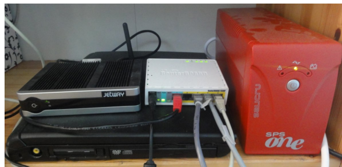
Figure 2.4: Indoor hardware of a community network node with router, server and cloud resource
