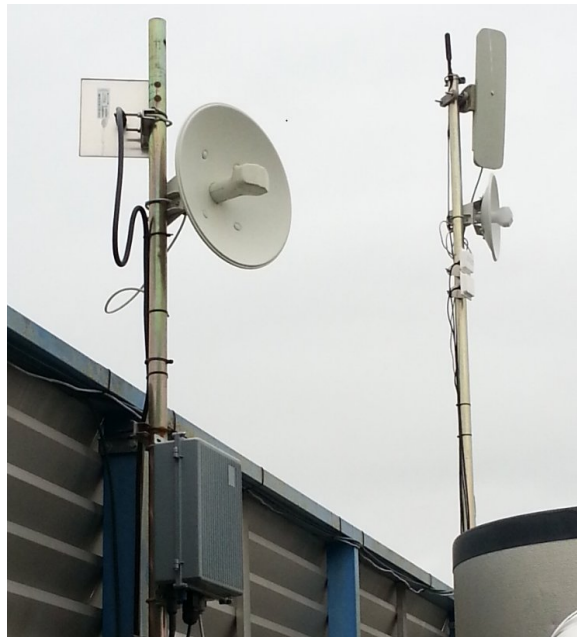
Figure 2.3: SN with outdoor hardware for wireless links
